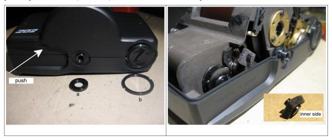
The viewfinder tower is not fixed with screws, so it may be easily removed
