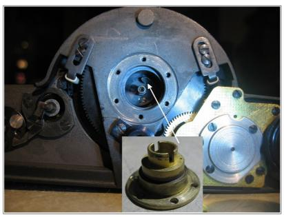
It is very simple, just enter the pin and turn it a bit left and right until it engages.
