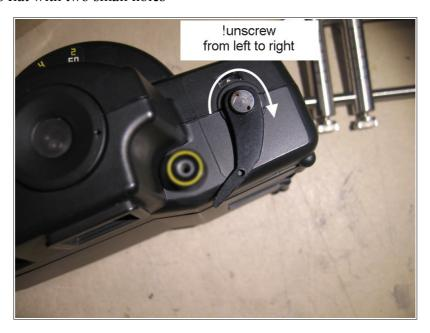
Unscrew the cylindrical screw under the cocking lever
