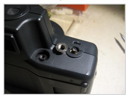
unscrew the shutter button, inside which there is a spring
