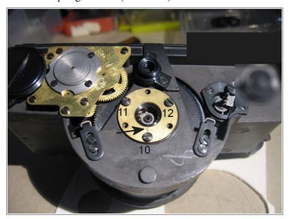
At this point stuck a screwdriver into one of the three holes without screw, whear a rubber glove and hold firmly the brass cylinder, then unscrew the three screws 10,11 and 12, always putting pressure against the brass cylinder, remove the screwdriver from the hole. The spring that is beneath the brass cylinder will turn from left to right. Let it run slowly and count how many laps it does (in my case about 3).
