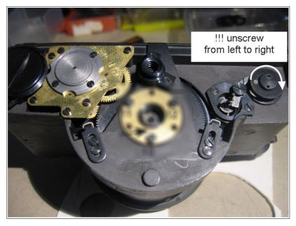
**Optical cylinder** (part above) (The shutter is always in the cocked position)
