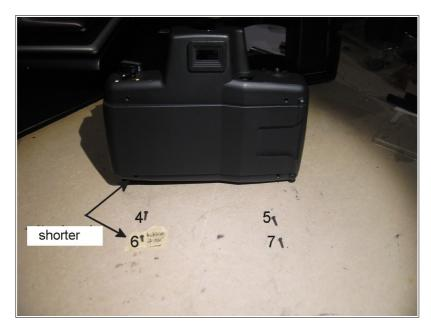
(Left figure) now for removing the back you need to rise the left edge and pry a little bit the frame while pushing it to the right (without bending the frame!) until the back is removed by interlocking with the screws that secure the camera door.
