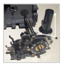
Place the nut holding the optical cylinder on the upper part of the camera and make sure that it locks well into place before tightening the screws 13, 14 and 15.
