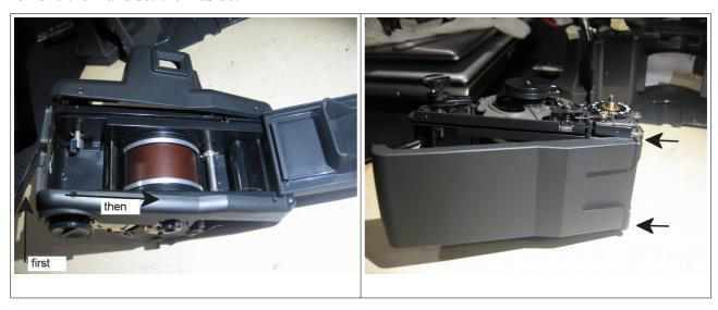
Before removing the screws 8 and 9 mark the outline of the metal tab, so that it will be easier to find the correct position later, then unscrew the screws 8 and 9 and slide out the tab.
