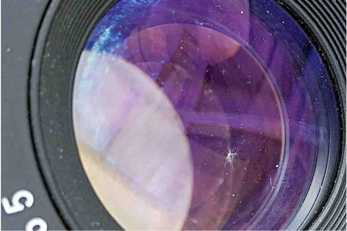
A closer look at the newly formed fungus in the 50mm f/1.8 E series lens.
