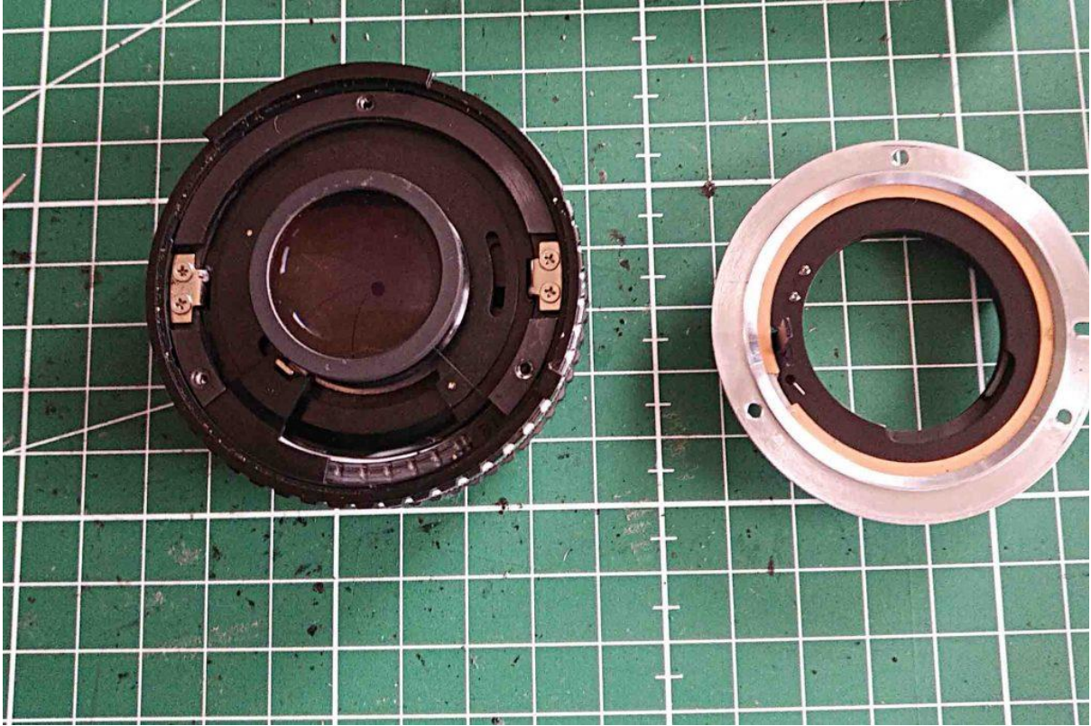
The bayonet removed from the lens, giving access to the back groups.
