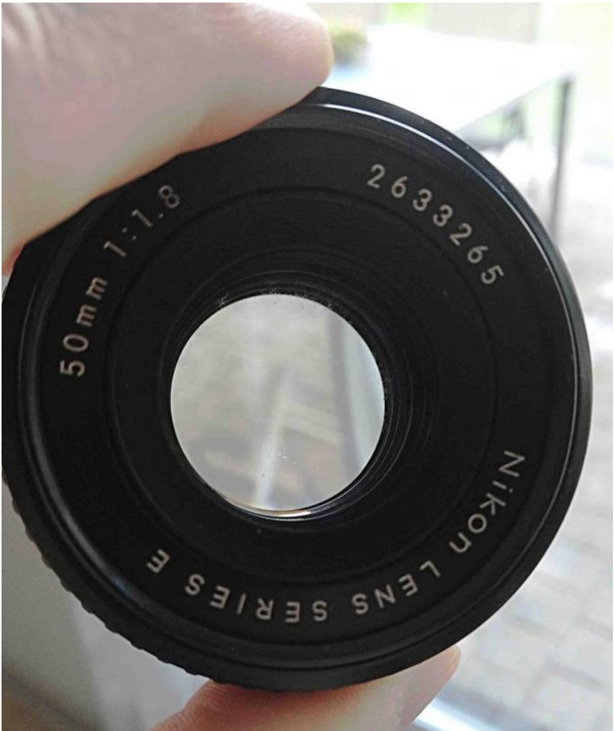
The front end is reassembled. The big spot of fungus has gone. What remains are traces of fungus in the back groups of the lens.
