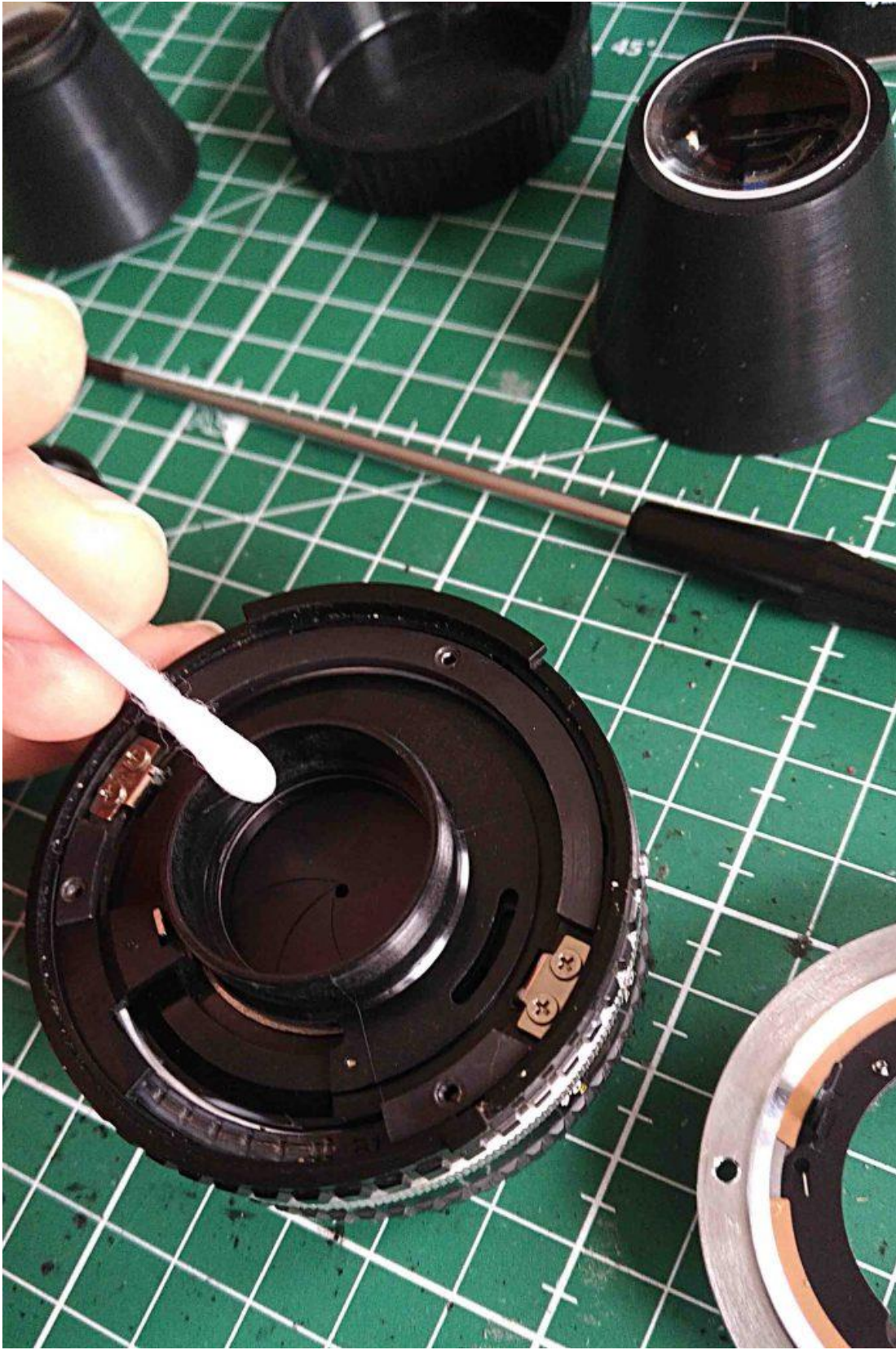
Cleaning of the lens assembly after extraction of the top lens from the one but final lens group. This lens is on top of the rubber grip.
