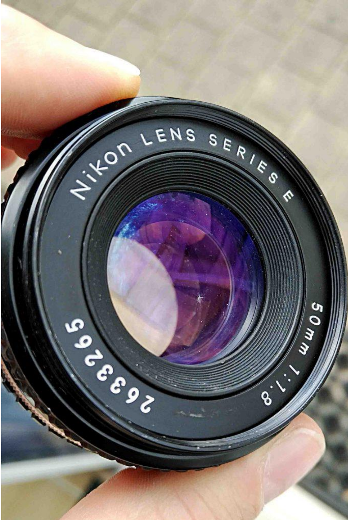
Cleaning of a Nikon 50mm f/1.8 E lens. The lens showing fungi on the internal lens elements.
