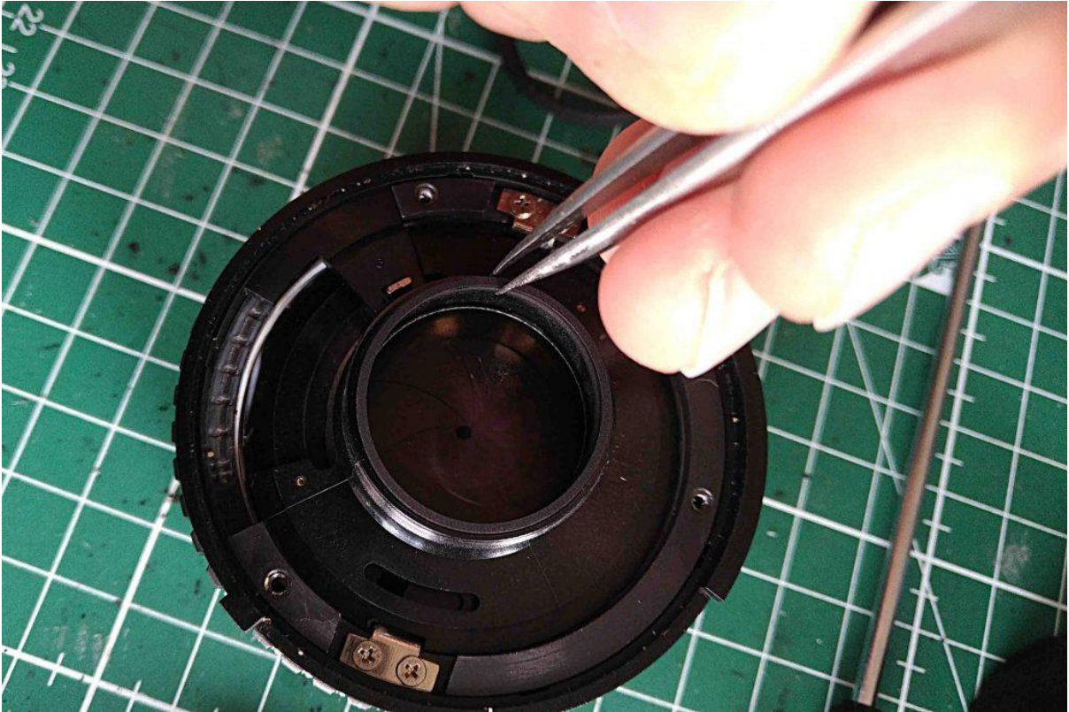
Removing the spacer between the last element and the last but final group.
