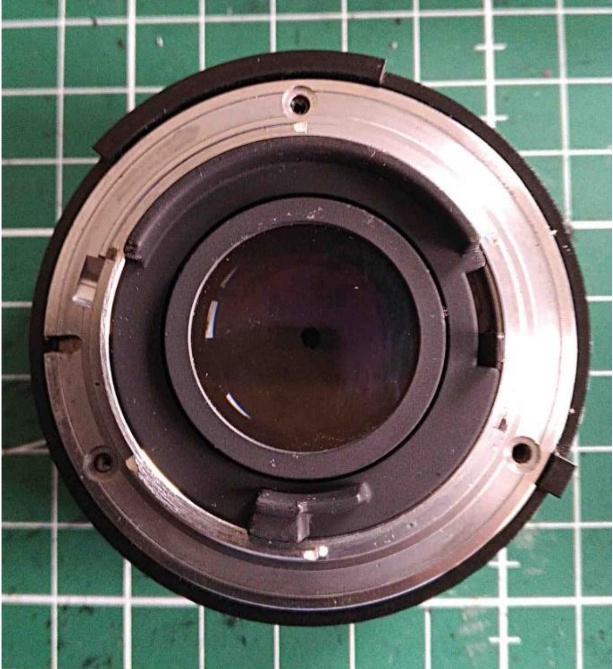
The three screws holding the bayonet are removed.
