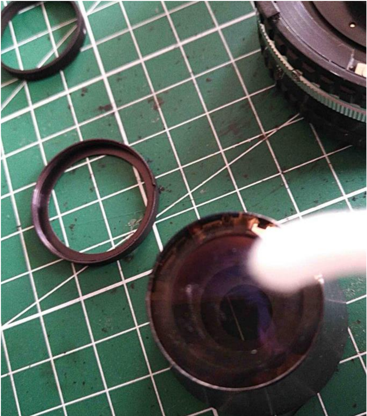
Cleaning lens elements, using hydrogen peroxide, water, alcohol and a carbon-tipped lens pen.
