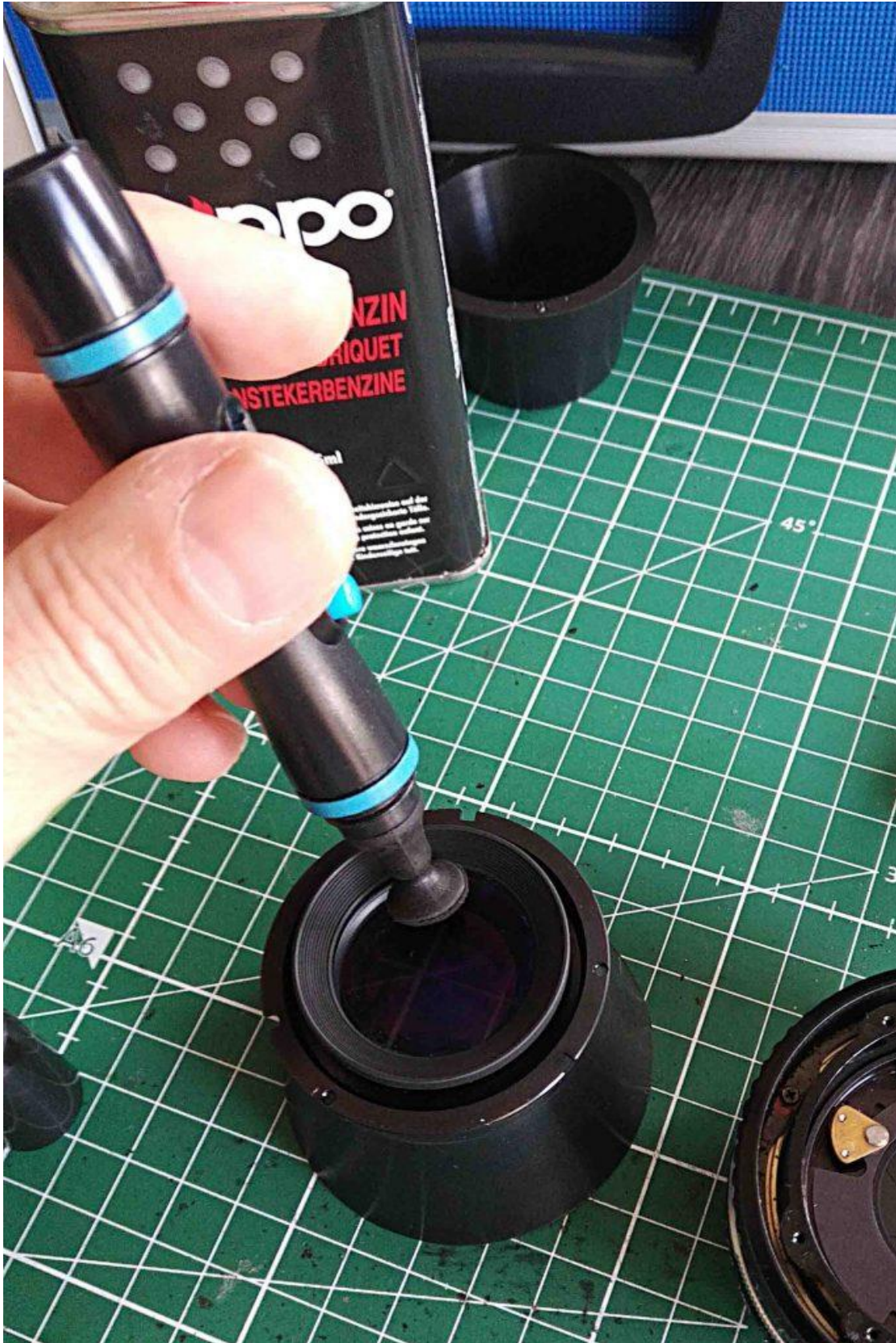
With a carbon-tipped lens pens we take away last grease traces on the lens elements in reassembling the front part.
