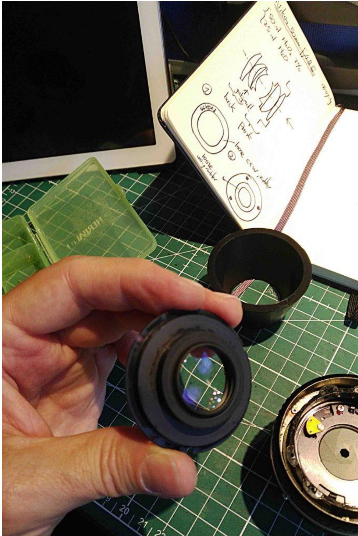
After removing the three screws, the second group can be taken out.
