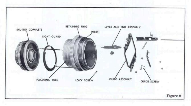
assembly, the focusing tube guide lug assembly, the two focusing tube guide lug screws, and the guide lug spring. If necessary, the focusing tube guide lug assembly can be disassembled from the focusing tube guide assembly by removing the two focusing tube guide lug screws.
