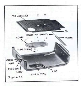
to push the window slide button through toward the outside of the back. Lift off the window slide.
