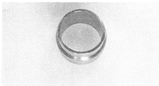
3650527 Use to hold 5th Lens Group in Tool No. 3650533 when centering Lens Group in Lens Group frame.
